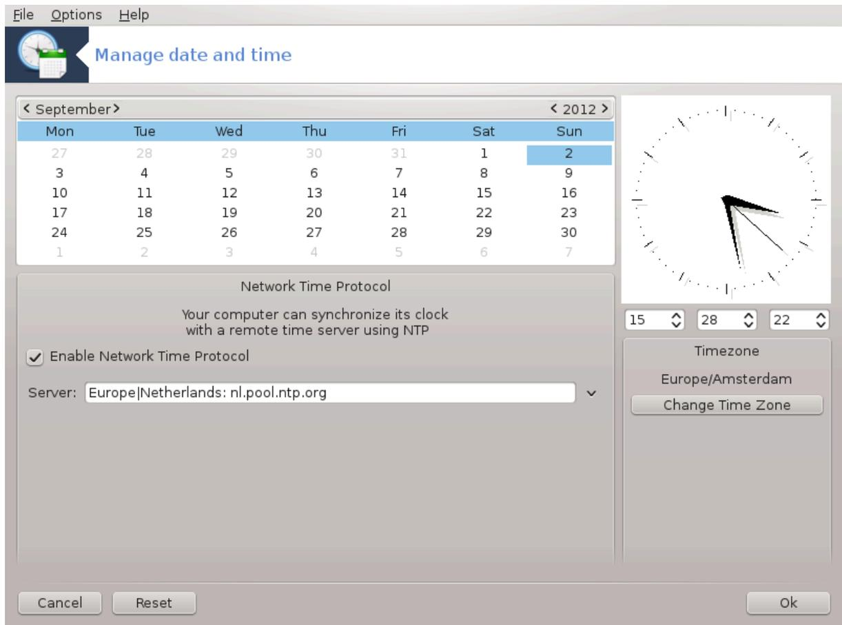
This tool<sup>28</sup> is found under the tab System in the Mageia Control Center labelled "Manage date and time". In some desktop environments it is also available by a right click / Adjust date and Time ... on the clock in the system tray.
