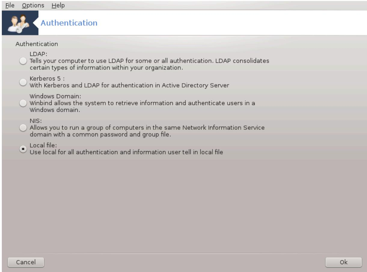
This tool<sup>26</sup> enables you to modify the manner in which you can be recognized as user of the machine or on the net.
