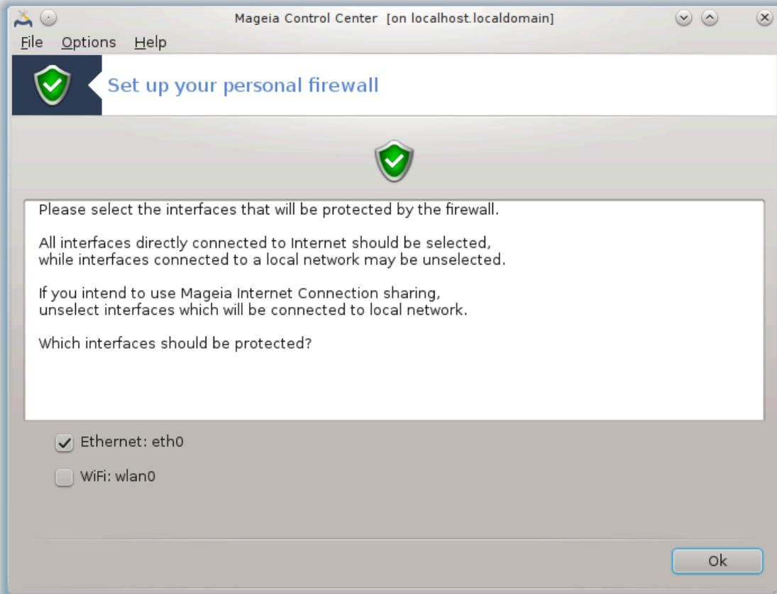
In the last screen, choose which network interfaces are connected to the Internet and must be protected. Once the OK button is clicked, the necessary packages are downloaded.
