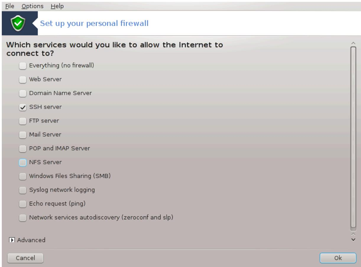
This tool<sup>44</sup> is found under the Security tab in the Mageia Control Center labelled "Set up your personal firewall". It is the same tool in the first tab of "Configure system security, permissions and audit".
