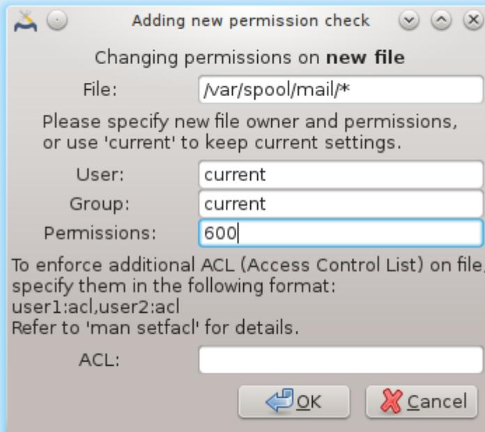
Click on the OK button to validate the choice and do not forget when leaving to save definitively your configuration using the menu File -> Save the configuration. If you have changed the settings, msecgui allows you to preview the changes before saving them.
