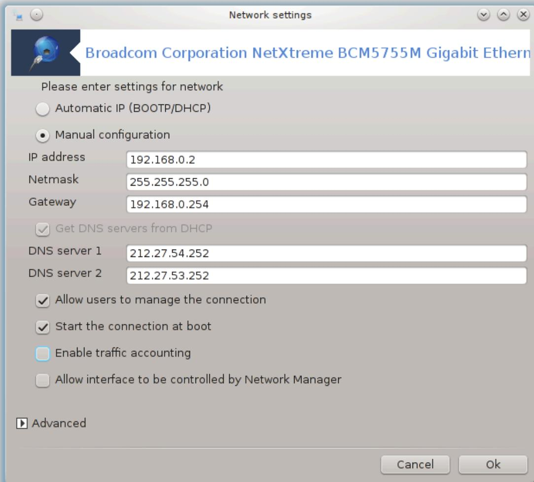
It is possible to change all the settings given during network creation. Most of the time, checking Automatic IP (BOOTP/DHCP) will do, but in case of problems, manual configuration may give better results.
