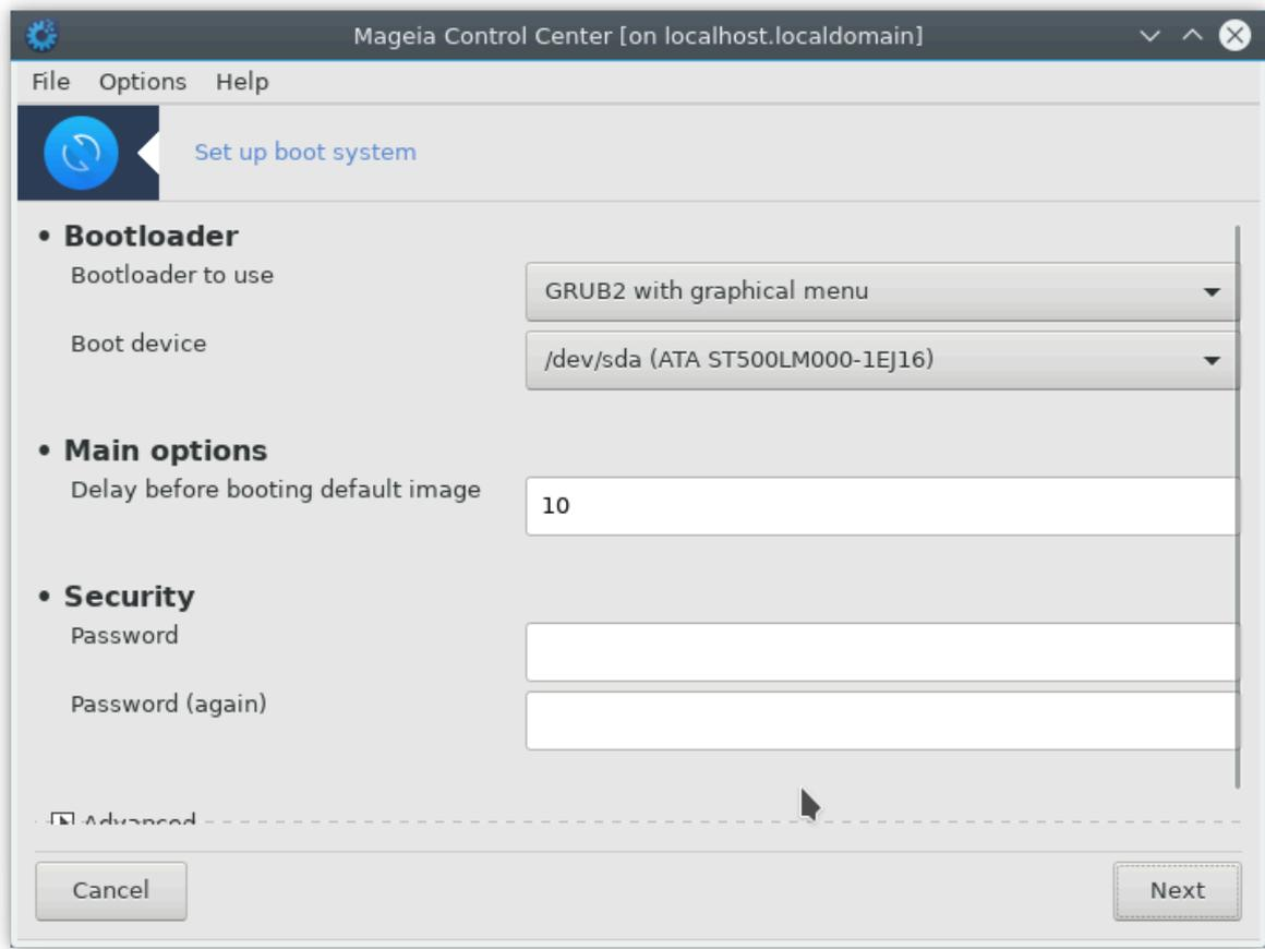
If you are using a UEFI system instead of BIOS, the user interface is slightly different as the boot device is obviously the EFI system Partition (ESP).
