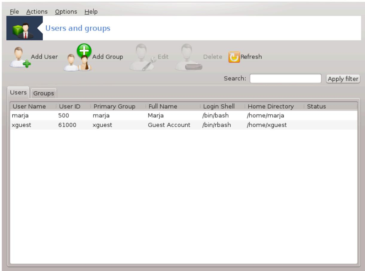
This tool<sup>32</sup> is found under the **System** tab in the Mageia Control Center labelled "Manage users on system"
