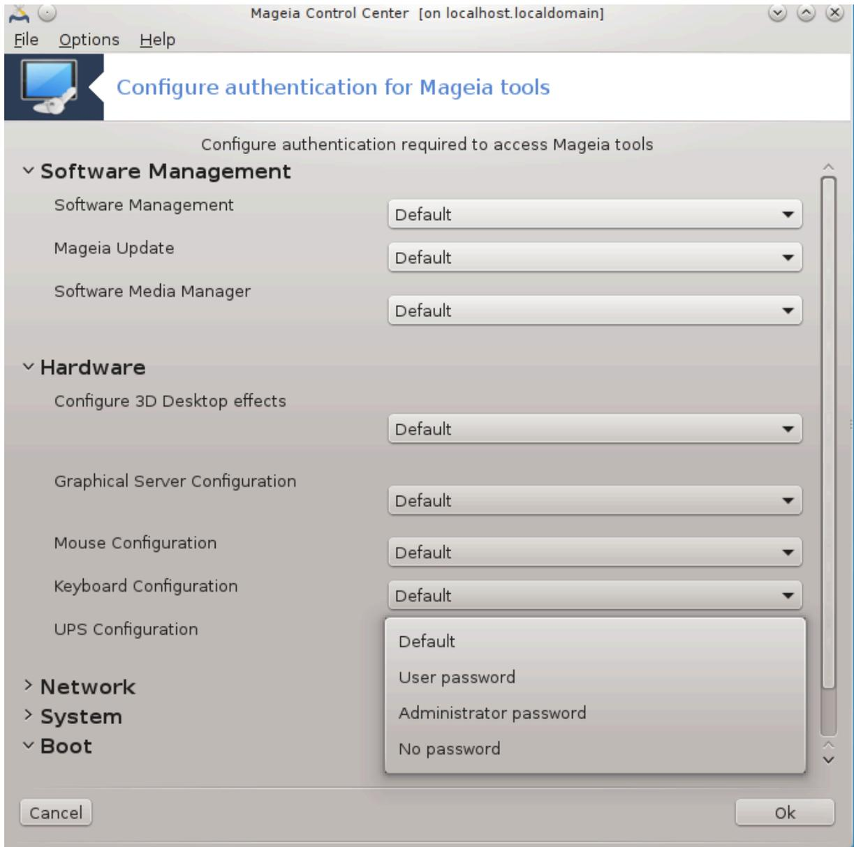
Most of the tools available in the Mageia Control Center are displayed in the left side of the window (see the screenshot above) and for each tool, a drop down list on the right side gives the choice between:
