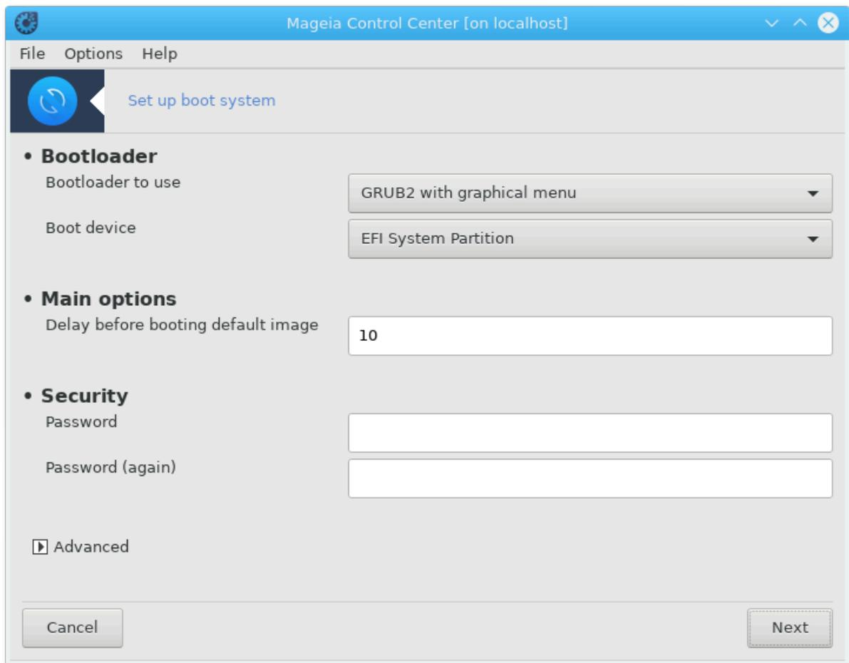
This tool<sup>48</sup> allows you to configure the boot options (choice of the bootloader, set a password, the default boot, etc.)
